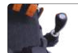
Single Joystick with Positive Locking System (Comfortable Positioning for Operation)
